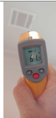
61 degrees observed at supply. 14 degree differential. Therefore evaporator coil is functioning properly.
